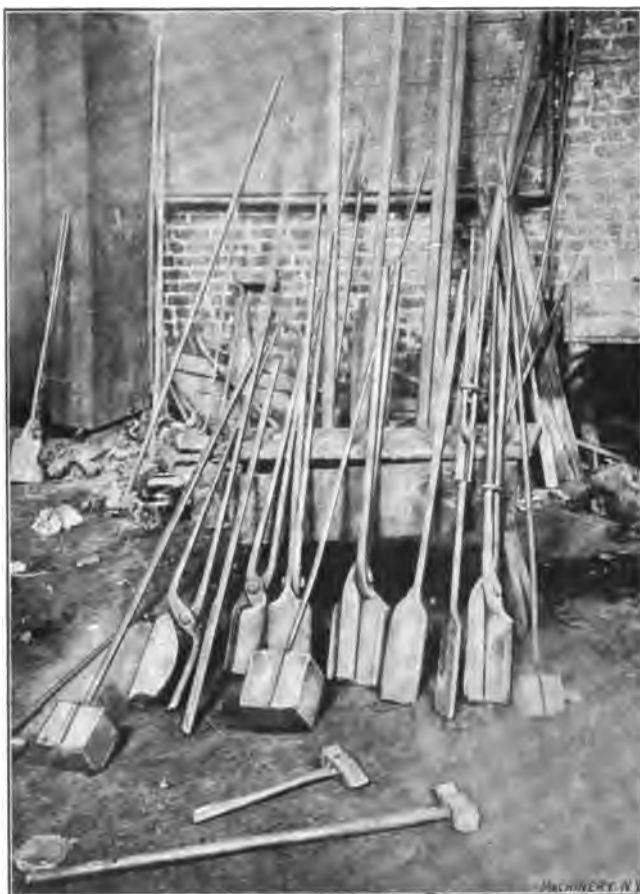
Fig. 4. A Collection of Tools used when Handling Crucible Steel Ingots and Hammering them to Size
